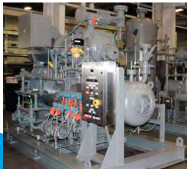
Ammonia compressor package Model 235S; 450 HP
