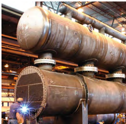
64" OD x 432" tube length flooded glycol chiller with 60" OD header
